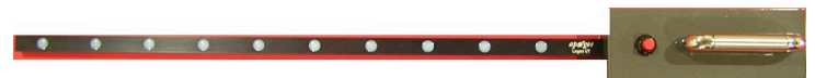
(An array of 10 PAR sensors embedded in a 1m long probe is used for large canopies / Tree)
