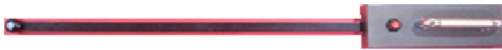
(1 PAR sensor embedded in a 0.5m long probe is used for small canopies)
