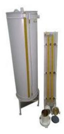
Soil Permeability Apparatus comes with glass tubes of 75mm, bore tube is provided with overflow arrangement for constant head tests. The remaining tubes are used for falling head test.
