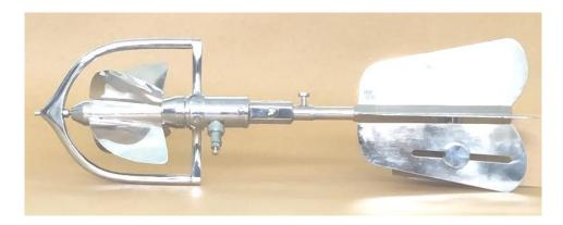
This "Virtual" make Propeller Type Water Current Meter is used to measure Velocity of water flow directly in m/s. The spindle carrying the propeller wheel freely rotates in the pivot assembly. The magnet and reed switch assembly produces one pulse per rotation. The rotation of the Water Current Meter is sensed by sensor & gives pulsed output signal.
