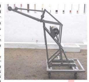
parapet or bridge sideway. It is capable of handling up to 100 kg. of hanging weight. Superior quality torque free wire rope from which the current meter is suspended is incorporated & wounded
